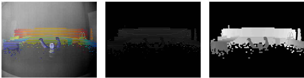
(a) Original point-cloud projected on the image plane. (b) Field-map image without interpolation. (c) Interpolation action on the field-map image.
