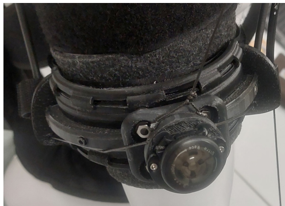
Figure 3.18 Shoulder slider guide and anchor point assembly demonstrating circumferential rail and bidirectional carriage.
