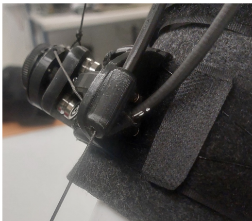
Figure 3.19 Elbow cable connector for intermediate routing guidance along upper arm.
