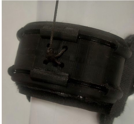
Figure 3.17 Elbow anchor point with cable termination.
