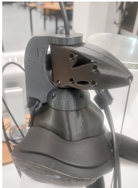
Figure 3.16 Mounting shoulder and cable director with cantilever mechanism.
