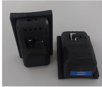
Figure 3.20 IMU Bluetooth modules: BMI085 6-axis sensors with Feather nRF52840 for wireless kinematic sensing.
