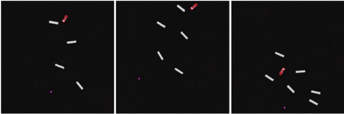
Fig. 4.9 Sample low-speed maneuvering environments, with different numbers of obstacles spawned with random positions and orientations.
