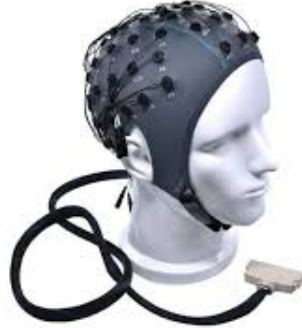
Figure 1.3: EEG cap with multiple electrodes.
