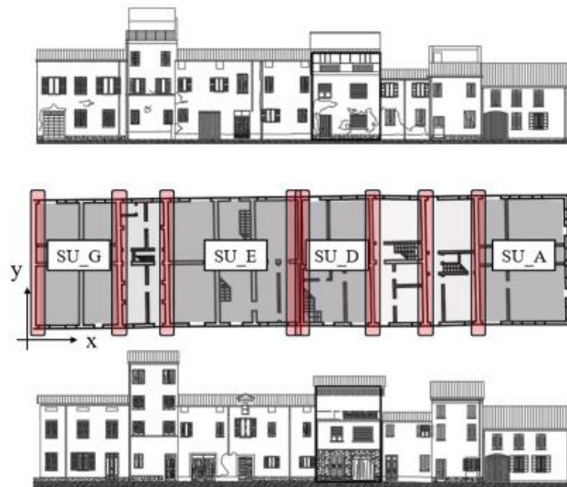
Fig. 1 Floor plan and elevations of the analyzed portion of the aggregate. The SUs analyzed both in the isolated configuration and within the aggregate are highlighted in dark grey. The walls without openings are highlighted in red.
