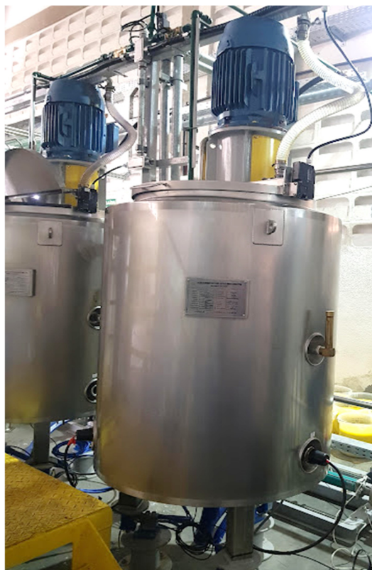
Figure 1. Homogenizing tank, with a capacity of 250 L, belonging to the biodetergent production pilot plant of the Advanced Institute of Technology and Innovation (IATI).
