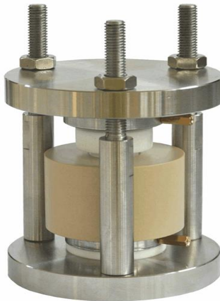
Fig. A3. 2 Image of test bench setup for ASSBs.
