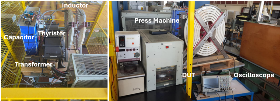
Fig. 4.6 Experimental setup used for measuring the forward voltage of the DUT across various surge current levels.
