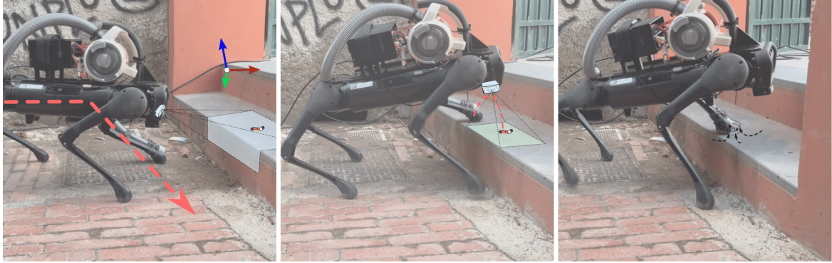
Figure A.4 Snapshots and illustrations detailing the collection procedure. From left to right: the system first detects the cigarette butt (CB) using the front-facing camera, and afterward, the planner defines a new optimal pose for collection (highlighted in the first snapshot by the coordinate frame centered on the hip of the robot's leg associated with the collection mechanism) deviating from the predefined path shown in red. Once the robot reaches the collection area, it utilizes the down-facing camera to refine the previous estimate of the CB's location. Finally, the robot proceeds to perform the collection by stepping on the target and activating the suction.
