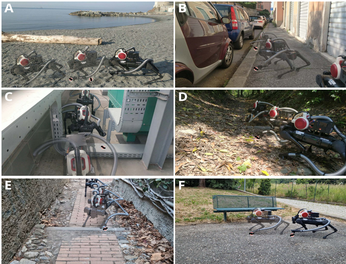
Figure A.7 The prototype has been tested successfully in six different scenarios. Starting from the top left corner, we show the robot, controlled with a joystick for safety reason, traversing environments named beach (A), urban (B), industrial (C), natural (D), non-flat (E) and park (F). All these scenarios are characterized by unique challenges both from the locomotion point of view, such as stairs and slopes (scenarios A, D, E, and F), and from the detection point of view due to the presence of similar objects in size and color (e.g. small leaves in scenarios D and F).
