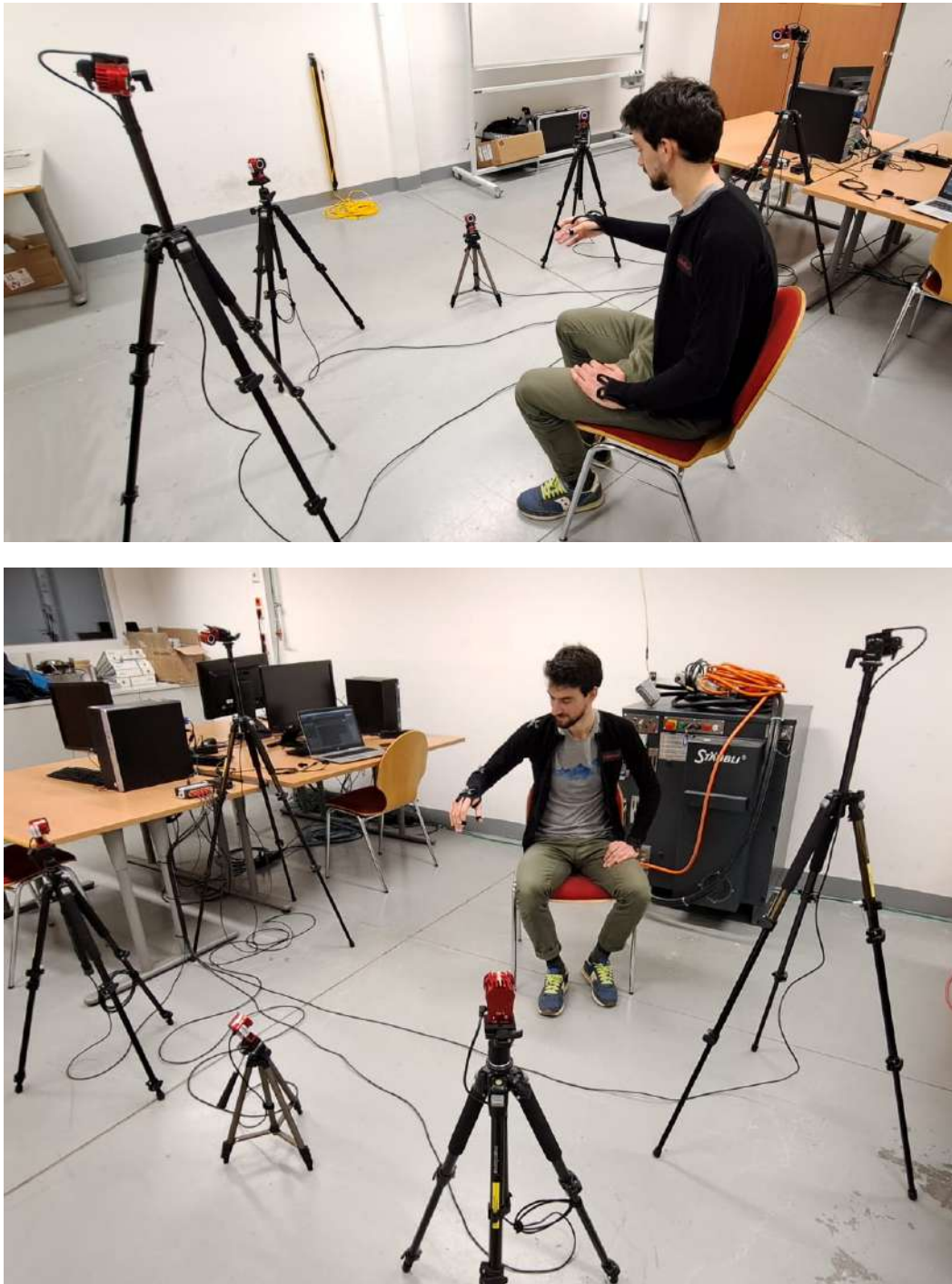
Figure 9.4 Overview of the setup of the tracking system.
