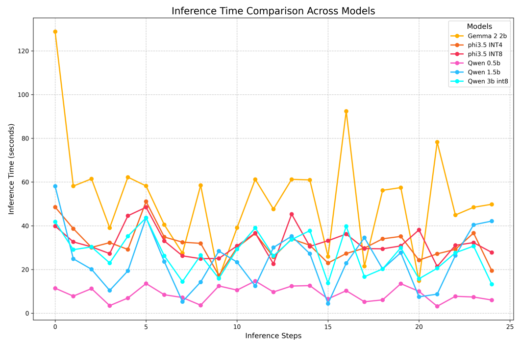
Figure 10. Comparison of the inference times for each question for the different SLMs.
