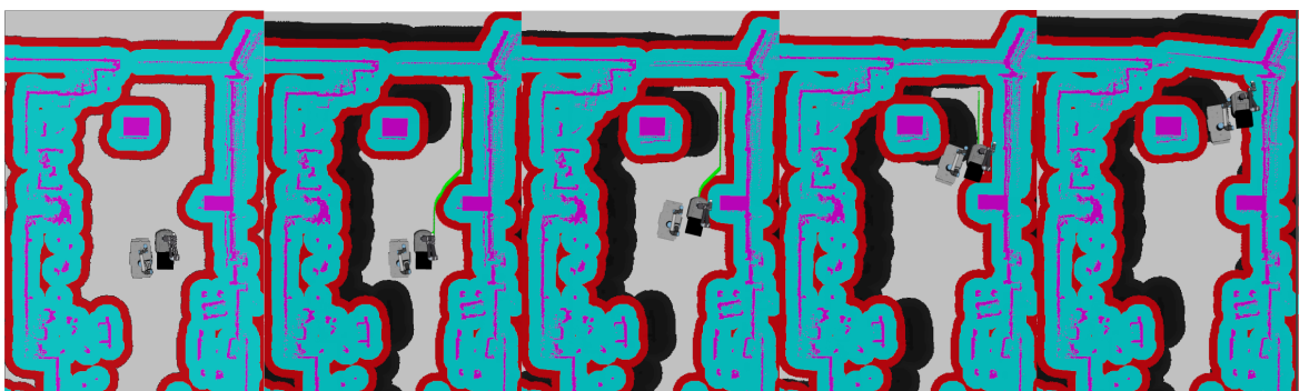
Figure 4.10 Visualization of multi-robot cooperative transport using RViz software. The most left panel shows the standard costmap computed by the leader robot. The remaining four panels show the execution of the test and the layer zero of the merged costmap
