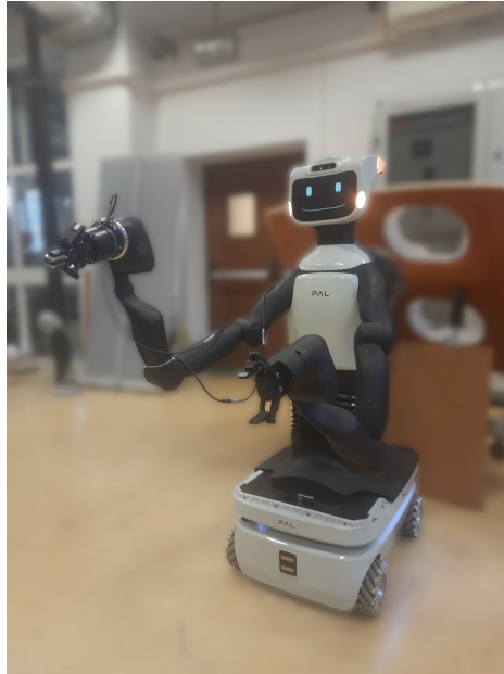
Figure 3.4 Tiago Pro used for the experiments, mounting Robotiq force-torque sensor and gripper
