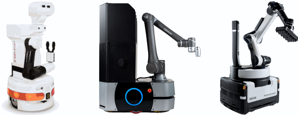
Figure 1 Examples of commercial mobile manipulators. From left to right: TIAGo from PAL Robotics, MoMa from Omron, Stretch from Boston Dynamics
