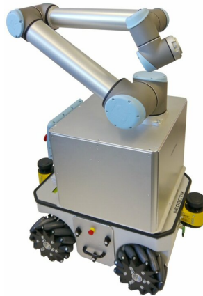
Figure 4.1 Typical example of an industrial mobile manipulator with a lightweight collaborative robot mounted on a mobile platform. (Credits to Neobotix)
