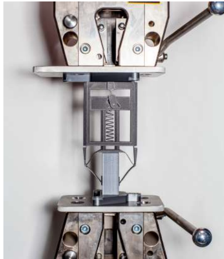
Figure 3.15 Experimental setup. The figure depicts the configuration used for the locking/unlocking tests.
