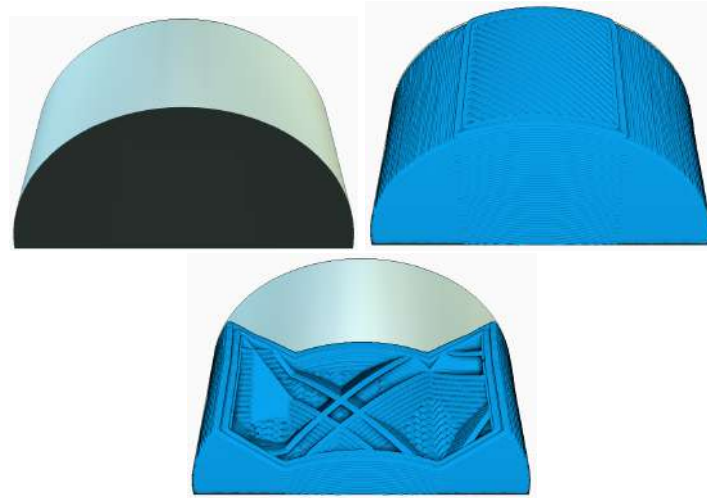
Figure 5.6 Top: Half a cylinder (left) and the trajectories produced by the presented technique (right). Note the curved top. Bottom: Showing half of the bottom layers (left) reveals the shape of the slicing surface (right).
