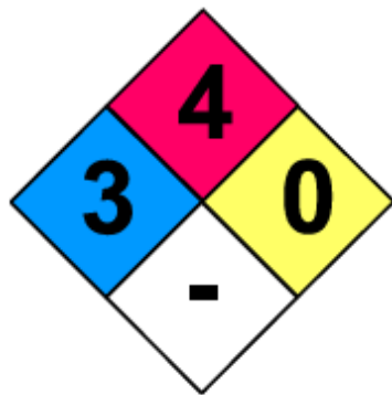
Figure 12: NFPA hazard levels for LH 2
