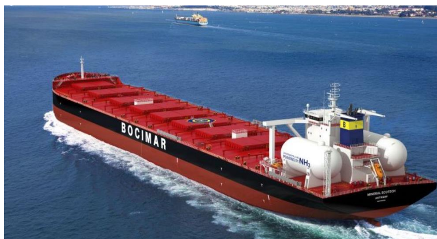
Figure 22: Possible storage tank arrangements on bulk carrier vessels
