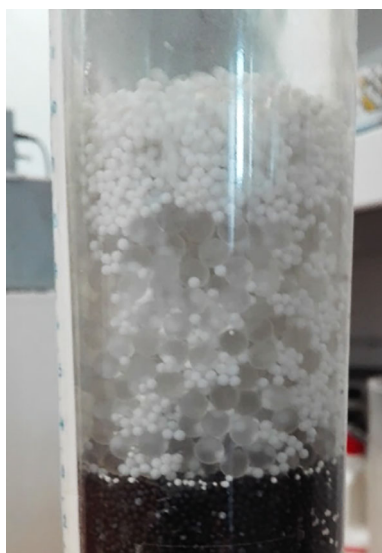
FIGURE 9 Picture of the binary-solid mixture 2.0TF + 4.9SG at a velocity intermediate between u_{if} and u_{ff} .
