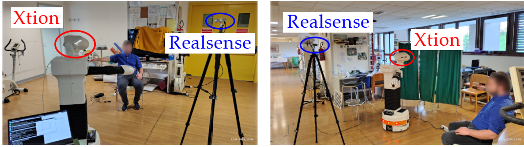
Figure 3.8 Final deployment for online mimicry, showing the two RGB viewpoints: TIAGo head camera (ASUS Xtion, used as reference optical frame) and an external Intel RealSense D455. Both sensors are RGB-D devices, but only RGB streams are used.
