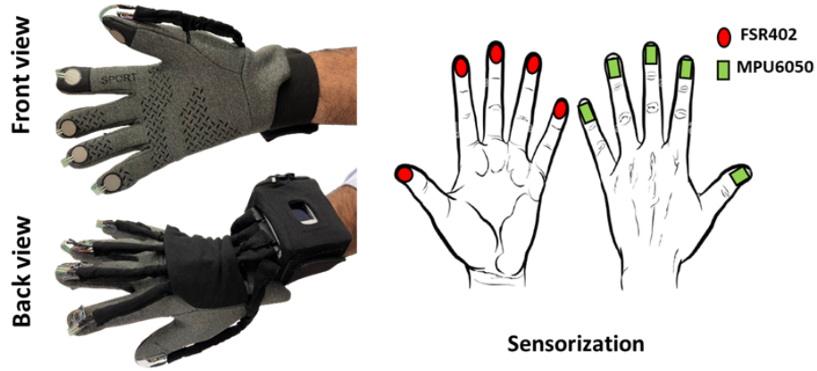
Figure 7.1: Front and back views of the developed multisensory glove, highlighting sensor locations.
