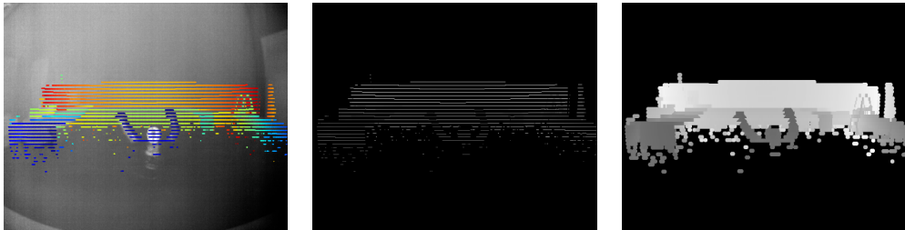
(a) Projected point cloud on the thermal image plane. (b) Range map before interpolation. (c) Range map after interpolation.
