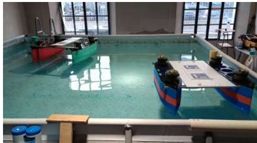
Figure 5.15: SWAMP vehicles performing cooperative four-corner test during the trials in the COMPASS lab.
