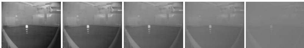
Figure 5.10: Fog augmentation with progressive Meteorological Optical Range decay.
