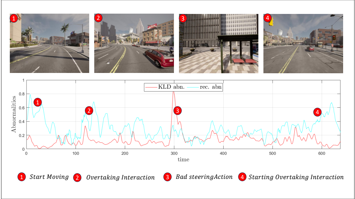
Figure 8.9: Explaining different sequences of actions in terms of anomaly signals. Online performance signal measured from the video latent state information. © 2024 IEEE.
