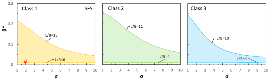
Fig. 5 Damping ratio vs. \sigma for the three structural classes considered, due to SFSI
