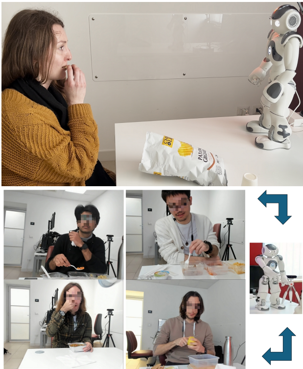
Figure 1: Top) The setup: the human is sitting in front of the NAO robot, eating the food, and having a conversation with the robot. Two cameras are used to record in sync the robot and human behaviors; bottom) Four participants during their interactions with the robot.
