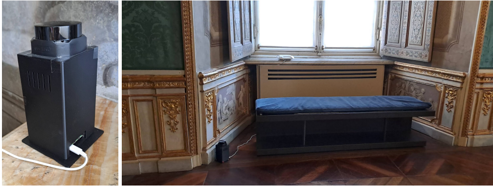
Figure 15.1 Left: a LiDAR device that was placed inside the museum to track the visitors. Right: one of the devices placed inside the museum.
