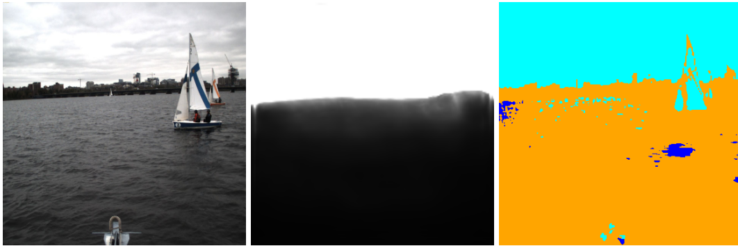
Figure 6.8 Sample predictions on MIT dataset using Co-SemDepth after adding custom augmentations. Depth is viewed in metric scale. Segmentation color index is: Blue=Sea, Cyan=Sky, Yellow=Ground/Buildings/Vegetation, Magenta=Other
