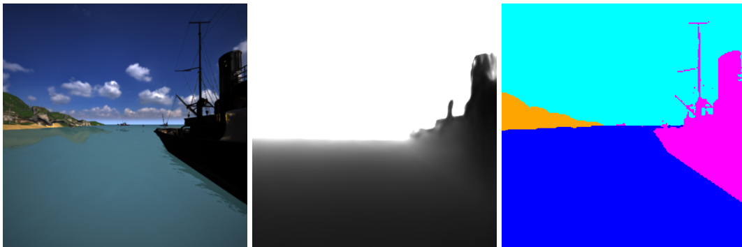
Figure 6.3 Sample prediction of depth and segmentation maps on MidSea. Depth is shown in a linear scale, and distance values greater than 255 meters are clamped to 255; that's why the far island disappears in the depth map. Semantic segmentation color index is: Blue=Sea, Cyan=Sky, Yellow=Ground/Buildings/Vegetation, Magenta=Other
