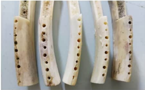
Figure 2. Ribs used for the evaluation of temperature changes (from top to bottom as position A, B, C, D, E, F, H)
