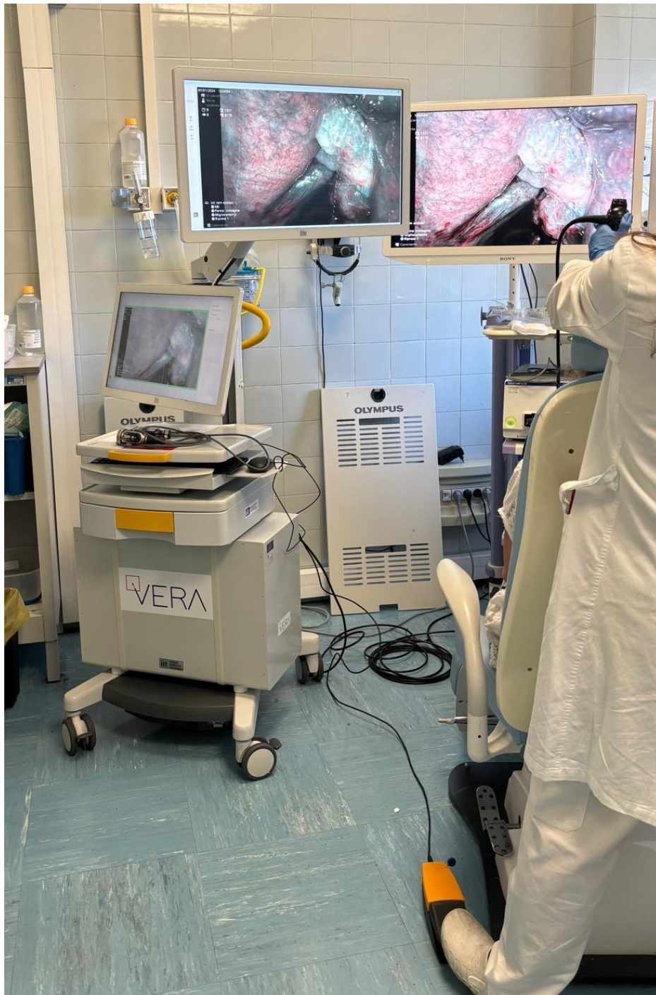
Figure 9.1 Illustration of the AI-assisted laryngoscopy prototype integrated into the clinical workflow. The interface displays a live endoscopic video feed on the top monitor and real-time AI outputs (bounding boxes of the detected lesions) on a secondary monitor not directly visible to the main operator. There is also a foot-pedal mechanism used by the operator for saving relevant frames.
