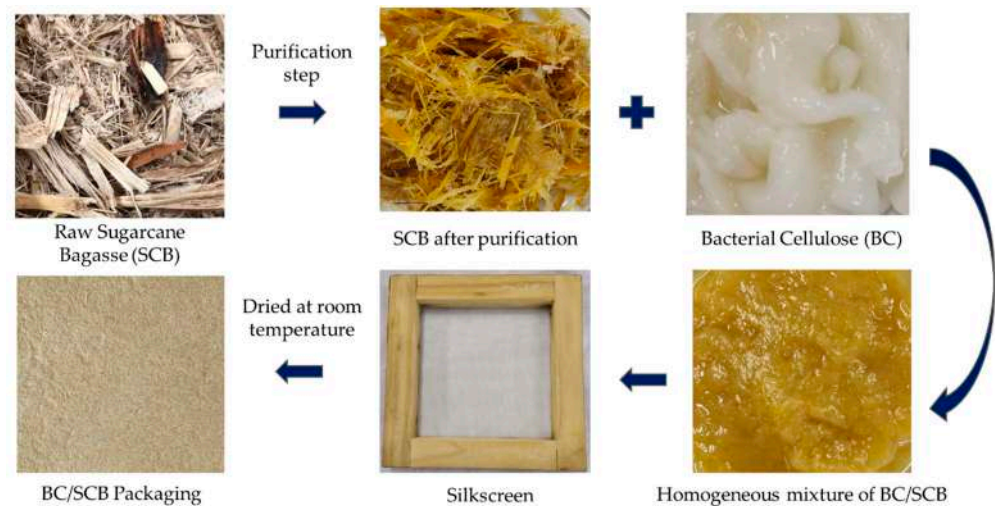
Figure 1. Scheme of production of bacterial cellulose (BC) and sugarcane bagasse (SCB) packaging material.
