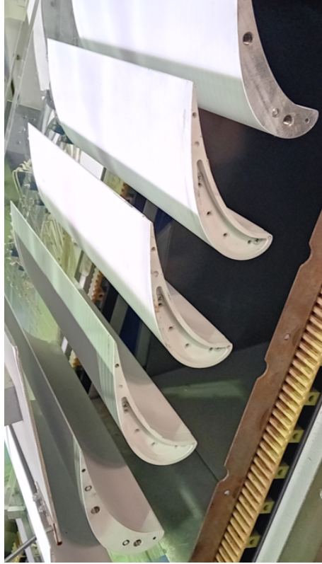
Figure 4.20: Unshrouded LPT cascade equipped with the squealer tip geometry on the blade tips.
