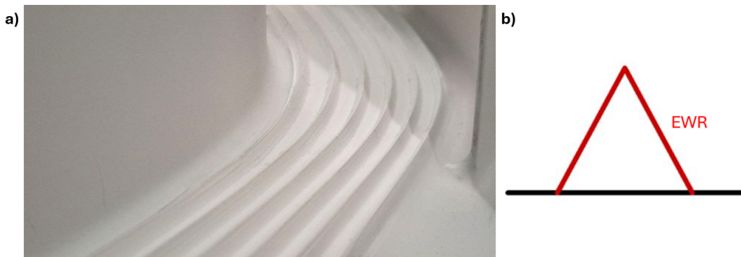
Figure 4.10: (a) Close-up view and (b) tangential section of the ridges on the NGV cascade endwall.
