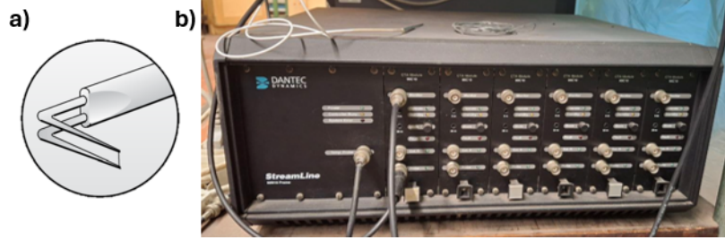
Figure 4.22: (a) Technical image of the probe and (b) CTA module.
