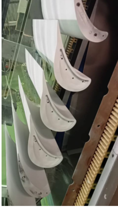
Figure 4.21: Unshrouded LPT cascade equipped with the squealer-winglet tip geometry on the blade tips.
