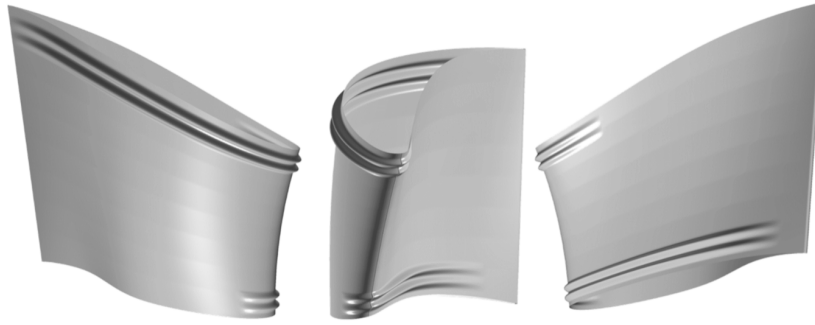
Figure 4.6: Example of blade fences in a 3D annular NGV.
