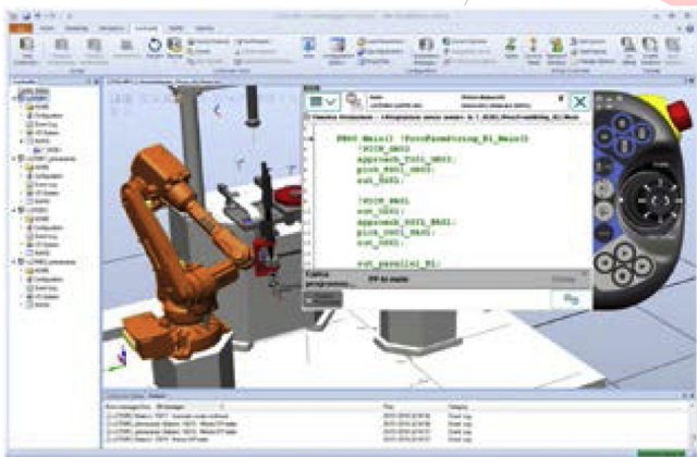
Fig. 3. ABB RobotStudio with its Virtual FlexPendant, [15].
