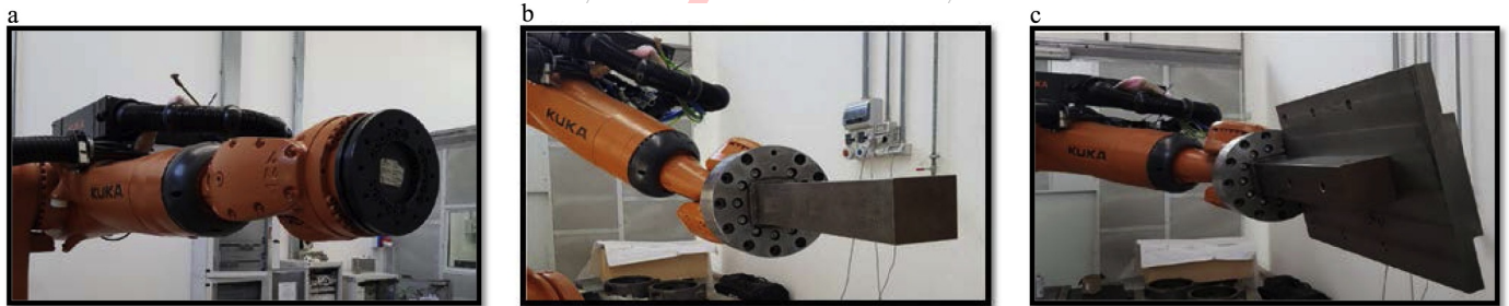
Fig. 15. (a) Load Type 1: no additional load applied on the IR end effector. (b) Load Type 2: beam with uniform cross section mounted on the IR end effector. (c) Load Type 3: beam with uniform cross section mounted on the IR end effector.
