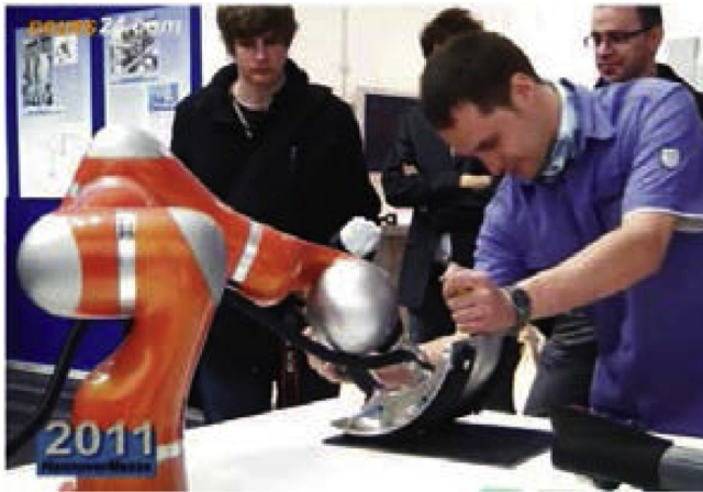
Fig. 1. Hand guiding programming for collaborative IR, [37].
