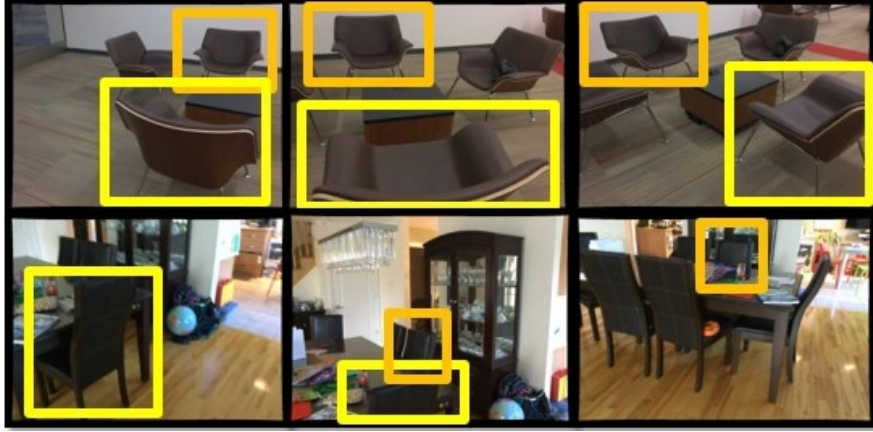
Figure 3.1: Similar looking objects in rigid, indoor scenes from ScanNet dataset. Multiple instances of the same object class, chair, in this case, are hard to differentiate with each other. In such cases, background can be highly useful to re-identify a particular instance in multiple views.
