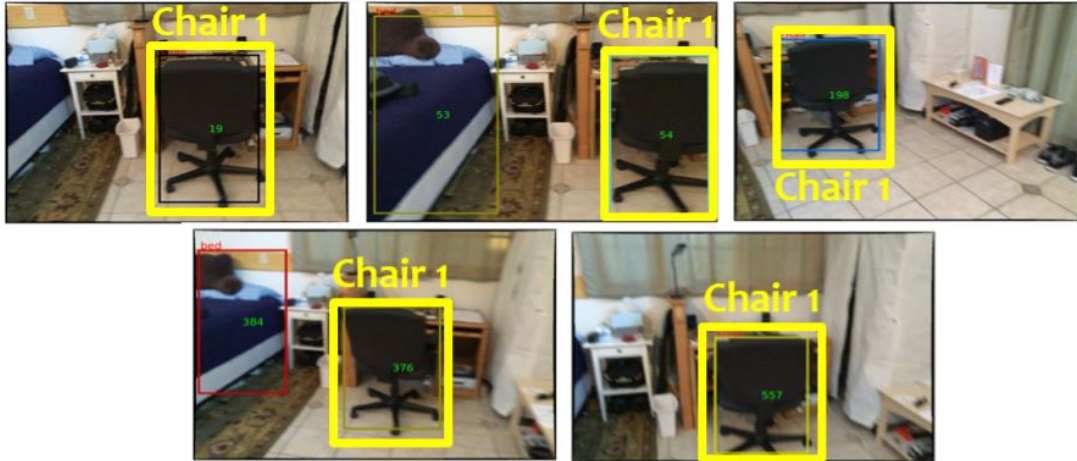
Figure 5.6: Multiple instances of the object class chair observed and correctly identified in different views. All these instances are now re-identified to be the same instance at different points in time.
