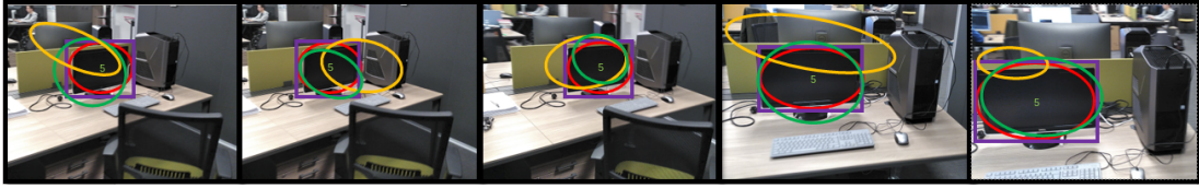
Figure 5.13: Once the object are detected, the bounding boxes are associated correctly across the multiple views we estimated the ellipsoids as shown in Figure 5.12. The ellipsoids are then back-projected on the images. The red ellipses in this figure are the ones fitted inside the bounding boxes for the detected object. The yellow ellipse are the projection of 3D ellipsoids generated with the poor association shown in Figure 5.10. The ellipses shown in green color are the projection of the 3D ellipsoids generated after the corrected association of 2D bounding boxes in the images achieved by using re-OBJ method.
