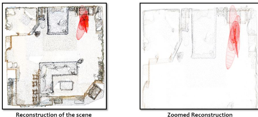
Figure 5.5: Reconstruction of the scene obtained from the ScanNet dataset [7] mapped with the 3D quadrics representing detected objects in the scene estimated directly by the 2D detections as explained in Chapter 4. Since, from Figure 5.4 we could see that the 2D detections across the images have not been associated as a result of which the 3D quadrics are not estimated accurately (seen on the right in a zoomed version)
