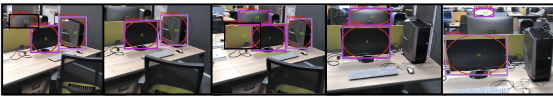
Figure 5.9: The objects are detected in multiple views using an off-the-shelf object detector such as YOLO [14]. The bounding boxes are fitted with 2D ellipses for the estimation of 3D quadrics as explained in Chapter 4. The bounding boxes are then tracked and associated across the multiple views. This example shows how similar appearances of objects of different categories or multiple instances of the same object category might lead to poor data association.
