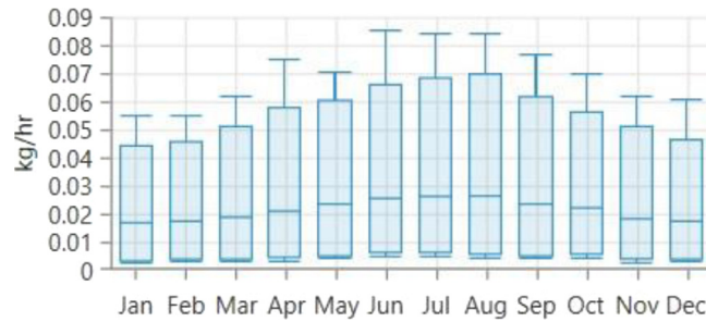
Fig. 10. Hydrogen consumption from the electrolyzer. Source: Own elaboration.
