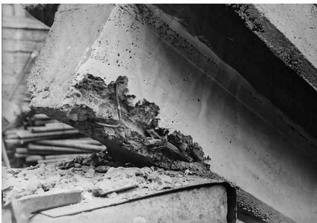
Fig. 3. Load test to collapse of a T beam performed by the Porcheddu company [27] - unpublished photo.
