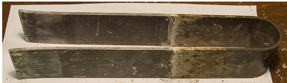
Fig. 22. Plate stirrup: deformed stirrup after the pull-out test.
