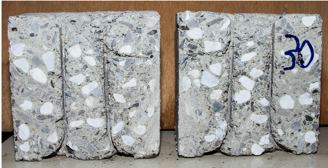
Fig. 23. Track left in the concrete cube by the plate stirrup. It is clear that almost no concrete crushing takes place around the stirrup.
