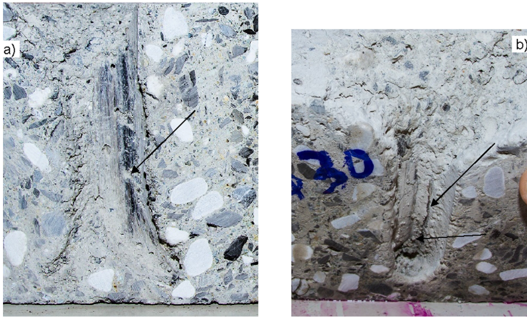
Fig. 21. Track left in the concrete cube by the fish-tail anchorage. a) sliding of the bar along the steel/concrete interface; b) the central track (black arrows) show the sliding and the side crushing of the concrete due to the two tails.
