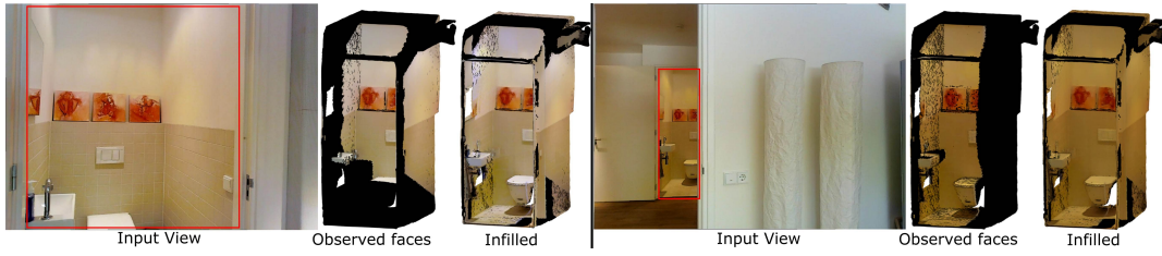
Figure 6.3: Mesh infilling: Two input views for the same scene, observed faces, and the result of infilling. The visible part of the scene is enclosed in the red rectangle. It is clear that there is a difference between infilled faces color degrees from the two views. Note: the black faces in the infilled part is for the faces which are not appearing from any view.
