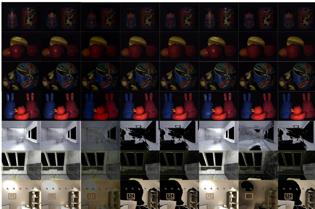
Figure 3.1: From left to right: Original image, Akashi et al [1], Lin et al [2], Souza et al [3], Shen et al [4], Tan et al [5], Yang et al [6], Yamamoto et al [7]. The performance of single images specular highlight detection and removal algorithms on conventional images used in evaluation (rows 1-4) which we can refer to it as lab-constrained images, and on normal images (rows 5-7), it is clear that they are performing good on the conventional used images but they have very poor performance on natural (non lab-constrained) images.
