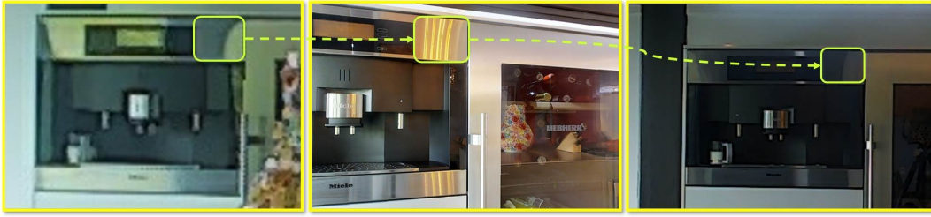
Figure 5.3: Three images of the same object from different view-points. The object part inside the green rectangle of the middle image is specular while other rectangles in other images contain diffuse reflections, it is obvious that the middle one has higher brightness level than diffuse ones
