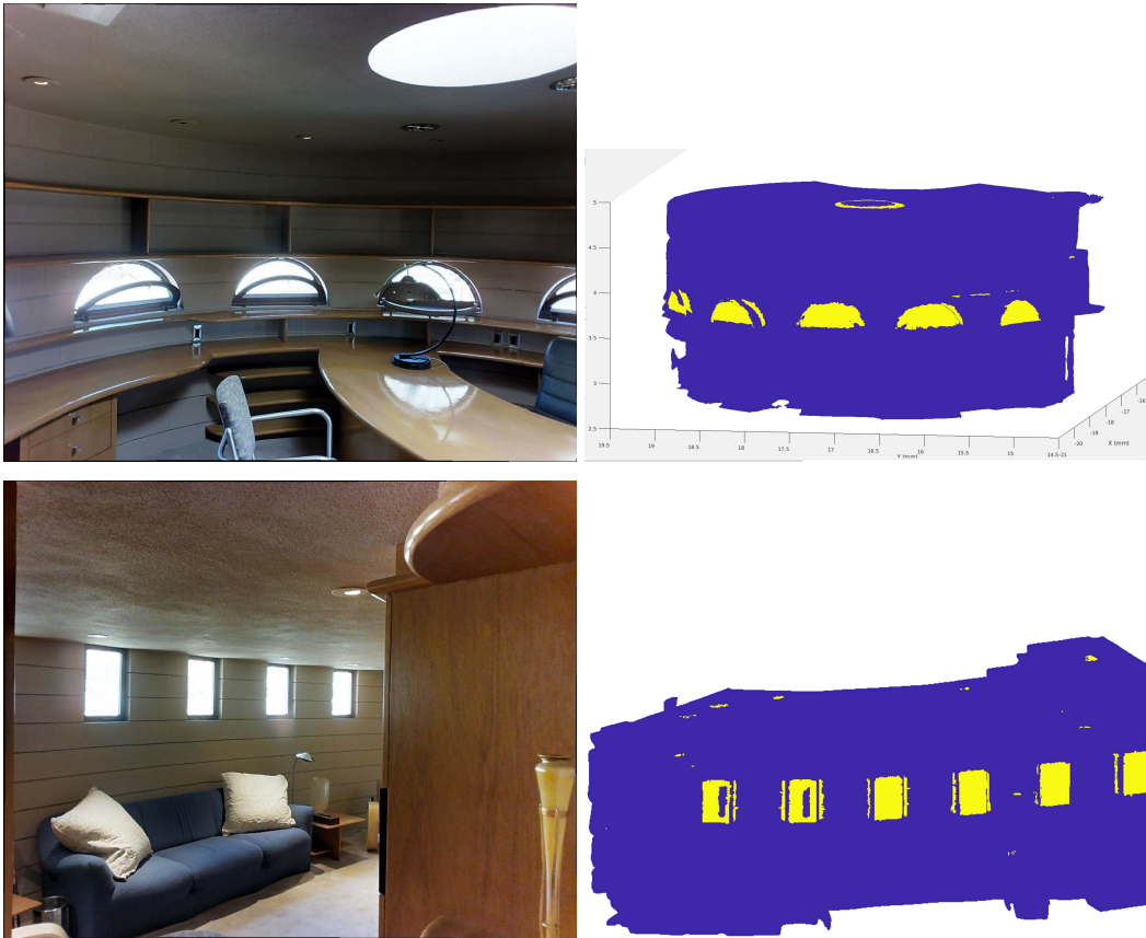
Figure 7.2: Sample from the M3DLS dataset, while the left column represents an original image from the scene showing some light sources, while in the right column our annotation (in yellow) projected on the 3D mesh (in blue).
