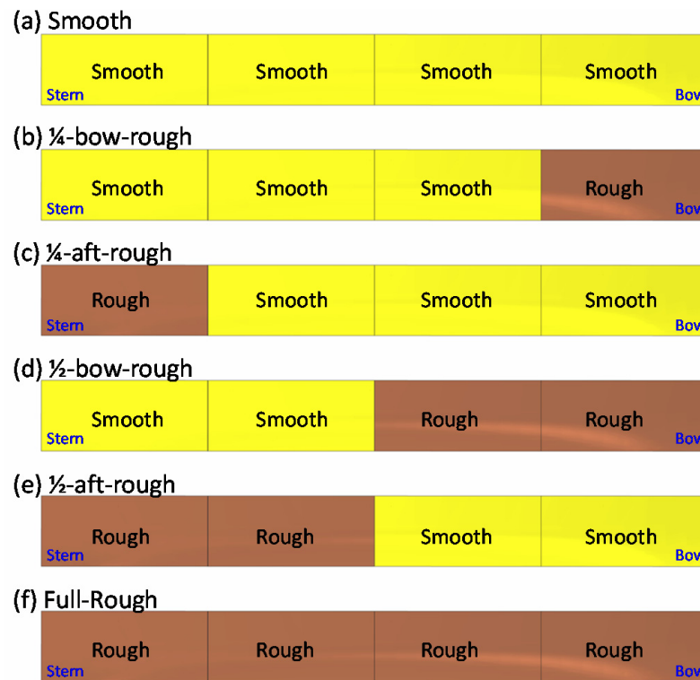
Figure 3. Different hull conditions of the Wigley hull simulations.
