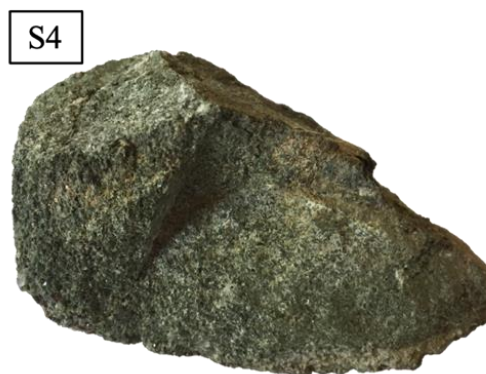
Figure 16. Close up photographs of analysed samples: S4, pyroxenite cut by talc and actinolite-filled vein.
