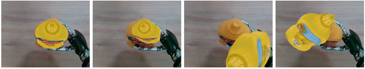
Figure 1.2 An example of robotic manipulation where a learning-based approach, DOPE (Tremblay et al., 2018), is used to estimate the pose of the bottle held in the hand of the robot. The estimated pose, that is superimposed on the input images, is not reliable and is characterized by discontinuities. Exploiting prior information on the interaction with the hand and alternative sensing modalities, e.g. touch, could help make the estimated pose more stable. The experiment was carried out by the author of this Thesis using the iCub humanoid robot platform.
