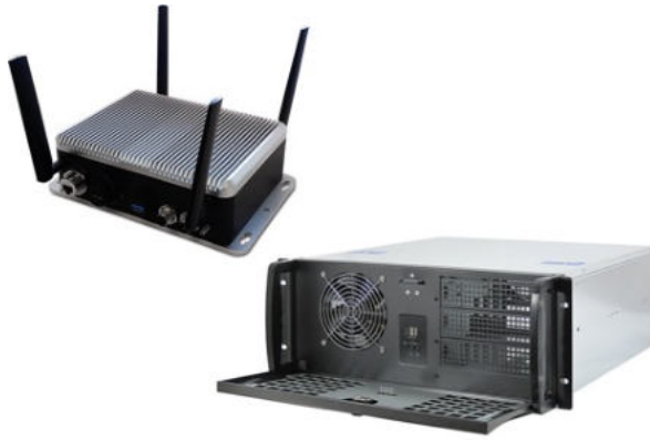
Fig. 7 Communication system (column gateway and RTU)
