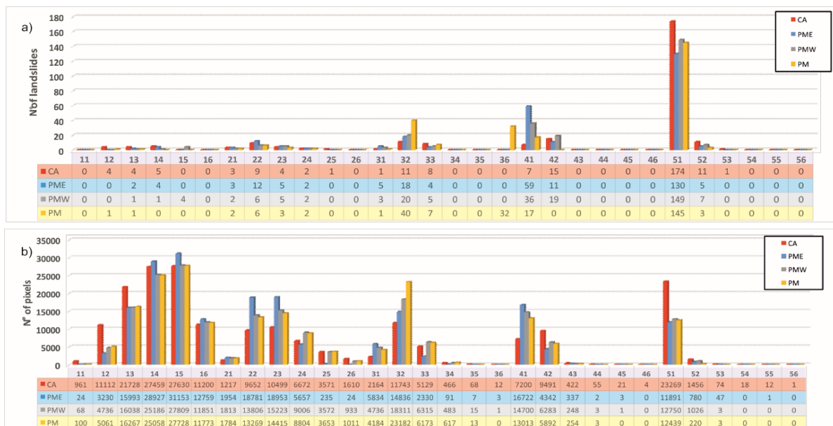
Figure 5.9 a) Graph resuming the results of the cross-comparison between landslides and each class of the confidence map; b) graph resuming the results of the cross-comparison between the number of pixels and each class of the confidence map.
