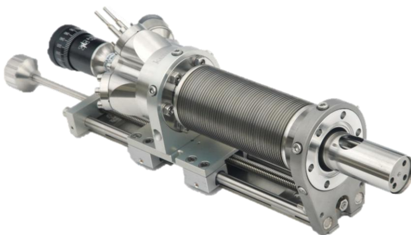
Figure 17: 4-cell UHV Evaporator TCE-BS by Kentax. Equipped with a z-travel unit and a corner- and gate- valve, four materials can be loaded and evaporated independently.
