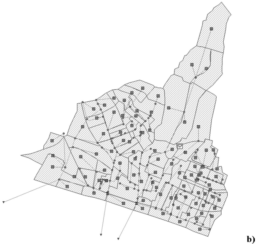
FIGURE 1 | (a) Overview of the case study area in the Sampierdarena district (Genoa, IT), drainage network (blue solid lines) and subcatchments' perimeters (black dotted lines); (b) EPASWMM model of the case study network.
