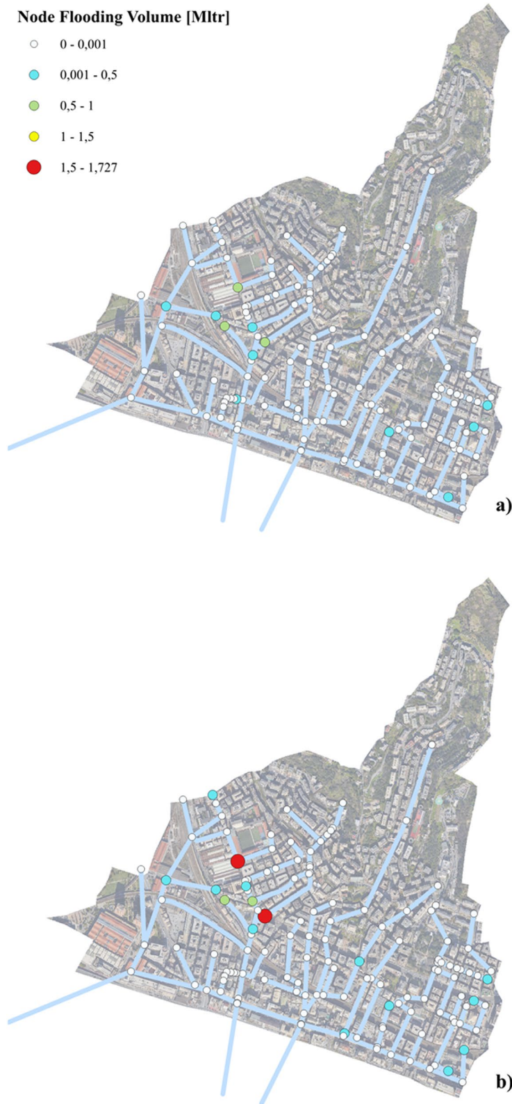
FIGURE 3 | Node flooding volumes in the Sampierdarena district (Genoa, IT) case study simulated for the current urban drainage system during the (a) 5-year and (b) 10-year return period rainfall events.
