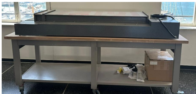
Figure 4-9 The above depicted tape caster is automatic, using motors to move the sheet at a determined speed and can provide heating from below to control the evaporation speed. As can be seen comparing it to the manual tape caster the dimension is much more like an industrial scale.
