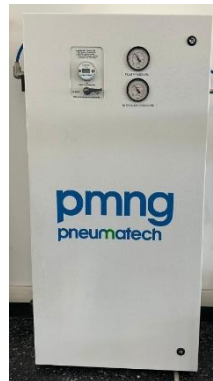
Figure 4-7 Nitrogen generator; on the left side the gas enters, the two gauges show firstly the input pressure of the air and the second one for the output pressure of the nitrogen.
