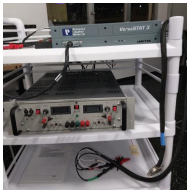
Figure 4-5 Voltmeter on top, that is connected to a PC for the reading, on bottom a booster module is attached, this is because the normal voltmeter is limited to a range of \pm 6V and \pm 2A , while the booster allows to reach \pm 40V and \pm 20A .
