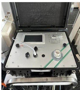
Figure 4-10 The IR - Spectroscopy in picture has both a small interface on the instrument itself and one that can be remotely accessed through ethernet connection. Importantly, the same rig as for the GC is used to clean the gases as also this instrument requires dry gases to avoid ruining the sensors.
