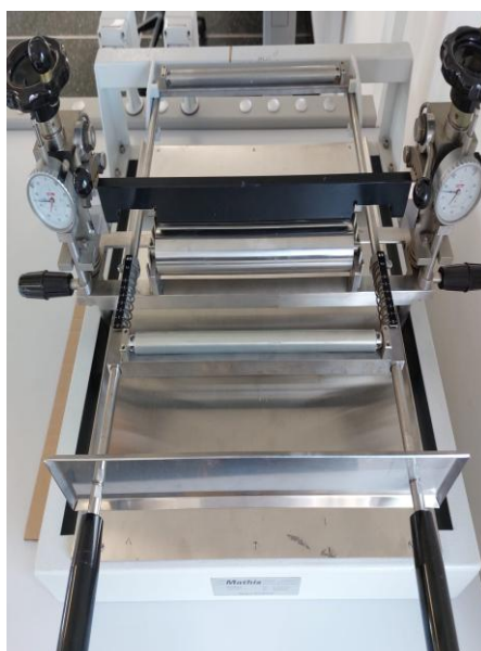
Figure 4-4 Tape caster; on top the black casting blade, on the sides the two height regulations can be seen, with their reading instruments. In the middle, under the blade the casting sheet should be stretched.
