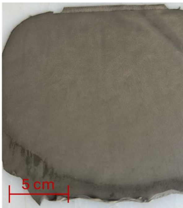
Figure 4-20 Electrode 4, produced through the new recipe. A slight phase separation can be seen in the bottom, but the middle part of the tape was looking good, smooth and without wrinkles.
