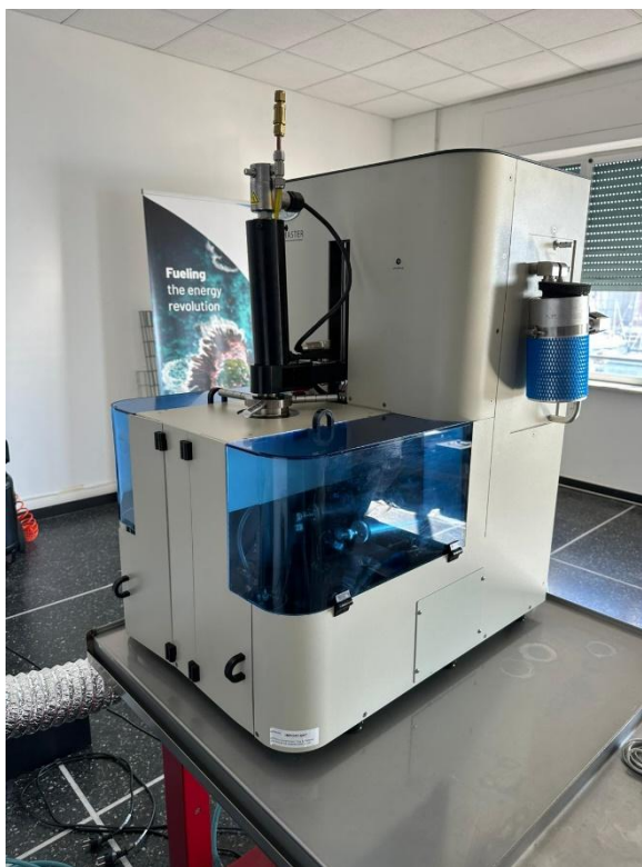
Figure 4-8 The mercury intrusion porosimeter, depicted in the accompanying figure, is equipped with two distinct testing modules to accommodate a broad range of pore size analysis.
