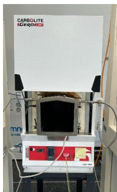
Figure 4-11 Controlled atmosphere oven; the external oven structure can reach up to 1200°C, while a reinforced chamber is inserted inside to allow for the formation of the controlled atmosphere.
