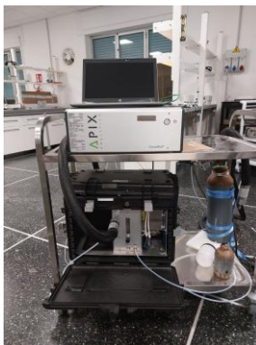
Figure 4-3 The GC setup is arranged on a two-tier tray. On the lower level, a condensation unit is installed to remove water vapour from the gas stream prior to analysis. On the right-hand side, a high-purity helium cylinder is provided as the carrier gas required by the GC and to maintain the appropriate backpressure. The upper level hosts the GC instrument together with the associated control unit and computer, which are used for instrument operation and data acquisition/visualisation.
