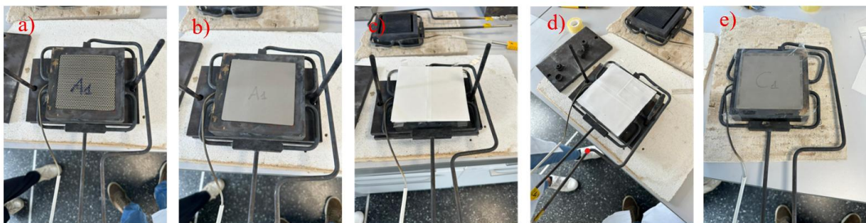
Figure 4-26 Cell setup in a 10 cm x 10 cm setup, from left to right we have a current collector (a), then the anode (b), then multiple layers of matrix and electrolyte powders (c + d), and in the end the cathode (e). Usually, the anodic side electrode is put on the bottom, and the cathode is on top.
