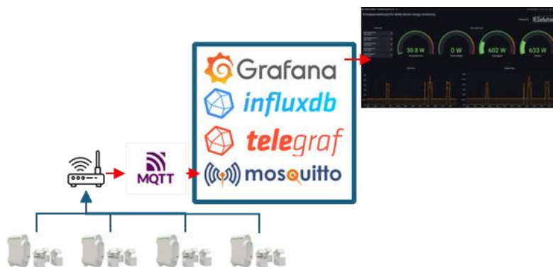
Figure 4.10 – Scheme of the ANTES monitoring system architecture
