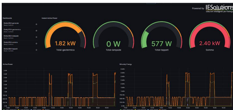
Figure 4.11 – Screenshot of the dashboard with general energy consumption data of the experimental greenhouse
