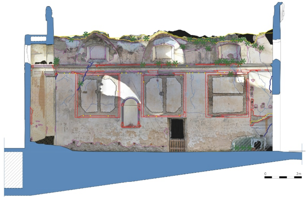
Figure 5. Map of the decay phenomena present on an internal wall of the oratory (elaboration by DAD, University of Genoa; scientific coordinators: R. Vecchiattini and S.F. Musso).
