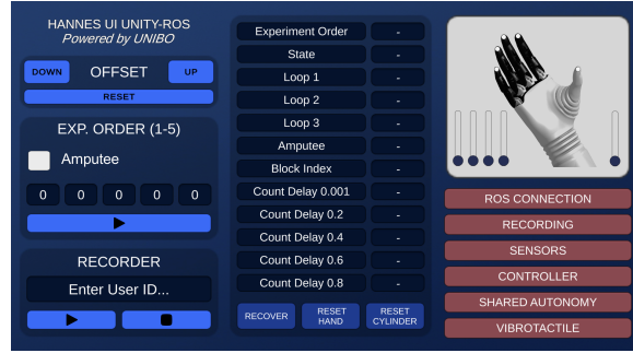
Figure 8.4 Researcher-side UI for the Intentional Binding protocol, with experiment-order controls, delay counters, reset actions, and system status/recording panels including hand visualization.
