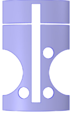
Figure 6.8: One of the ferromagnetic shields employed in the simulation. Image adapted from [84].
