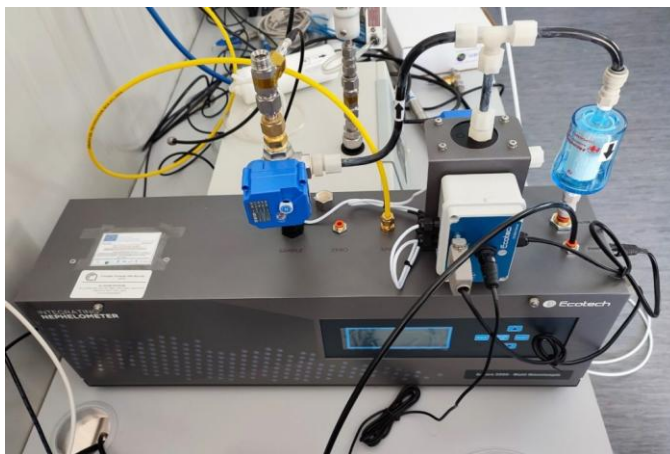
Figure 2.11: Ecotech Aurora 4000 integrating nephelometer used for real-time measurement of aerosol scattering properties.
