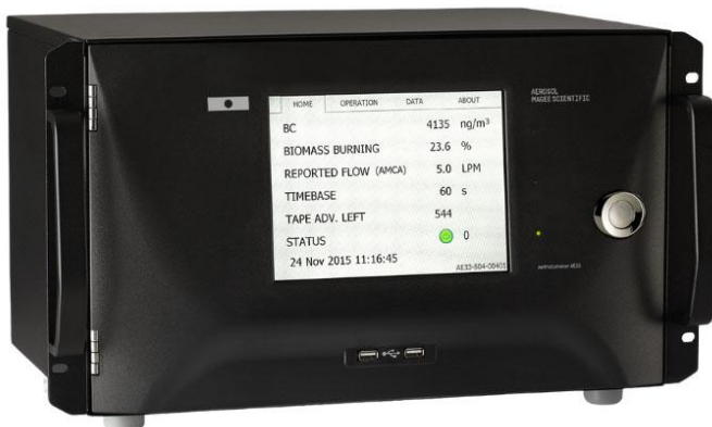
Figure 2.10: AE33 Aethalometer used for real-time measurement of aerosol light absorption and black carbon concentration.
