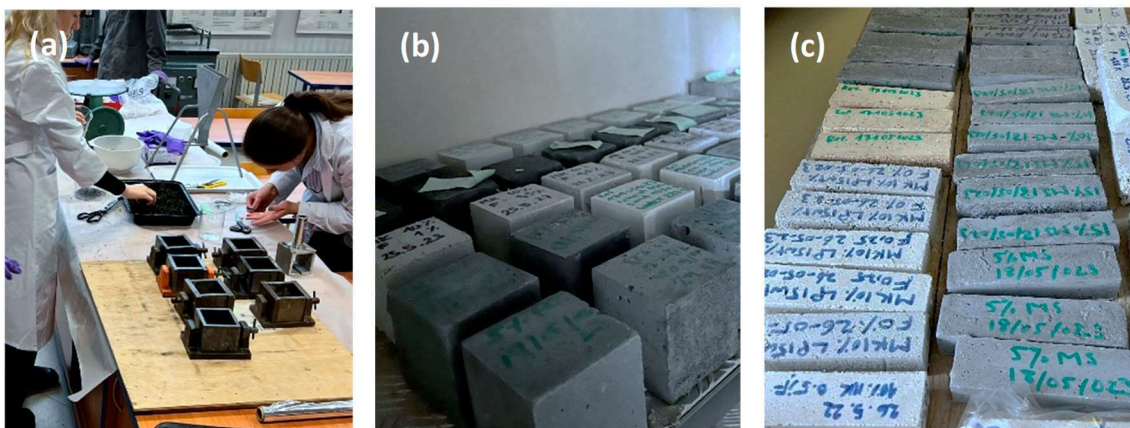
Figure 2. For each mixture, (a) cubical samples (70 mm × 70 mm × 70 mm) and rectangular samples (40 mm × 40 mm × 160 mm) were prepared, and (b,c) samples were cured under 98% relative humidity and 298 K for 28 days.
