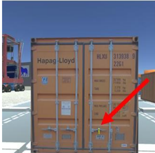
Figure 36. Door with Bolt Seal
