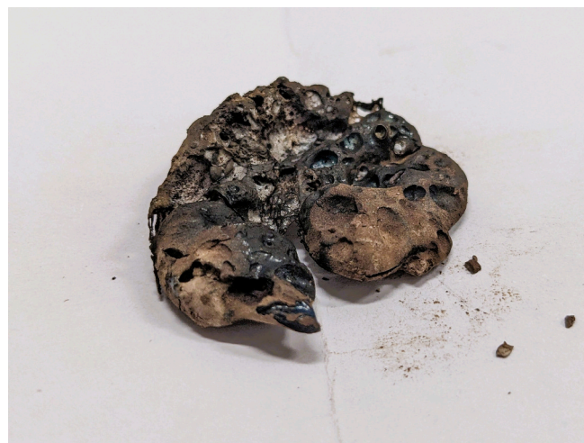
Fig. 9. The solid block recovered after the HTC of the MIX at 220 °C.
